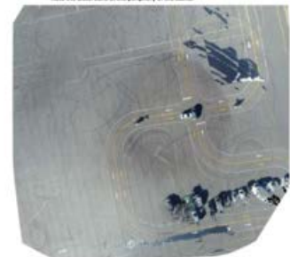
Figure 10-4. Orthorectified Orbit Trajectory at 19:00 from DJI Phantom 4 Pro with 50% (Day 1). Note the distortions at the periphery of the scene.
