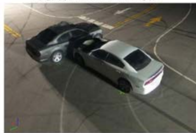
Figure 8-4. Close-Up View: 19:30 Two MLTs Orbit Trajectory from DJI Phantom 4 Pro (16-degree sampling) (Day 1). Note the artifacts on the roof of the gray car.
